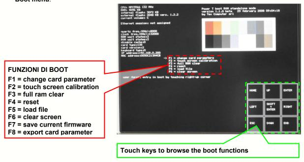
WARNING: the Boot menu only manages the USB memories and not any other peripherals, such as the keypad and the mouse, which may be connected to the same USB port by means of a hub.
