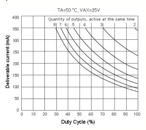
If the integrated circuit reaches the thermal overload threshold, all outputs are turned off; they automatically reset only after the internal temperature of UDN 2987 will have dropped by about 10%. During overcurrent shutdown the i22 output will remain at 0.
